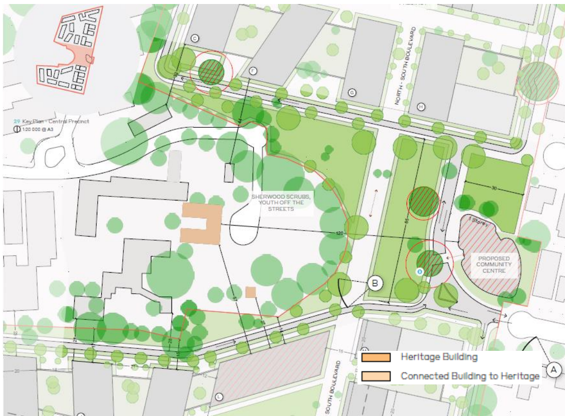
Figure 16: Proposed setbacks to buildings on the Sherwood Shrub site (Source: Ethos Urban)
