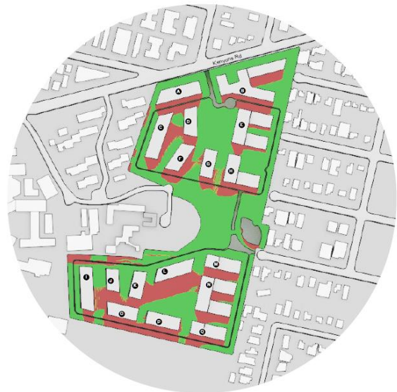
Figure 26: Solar studies of the indicative concept masterplan proposal against the ADG (source: Ethos Urban)
