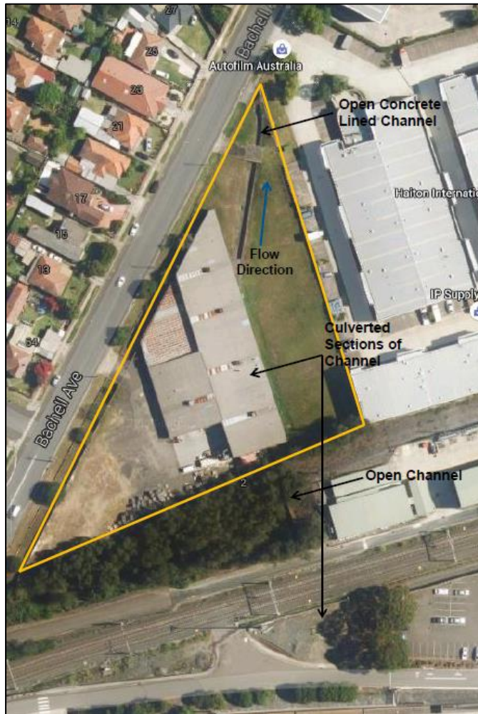
Figure 19: Existing drainage arrangement
