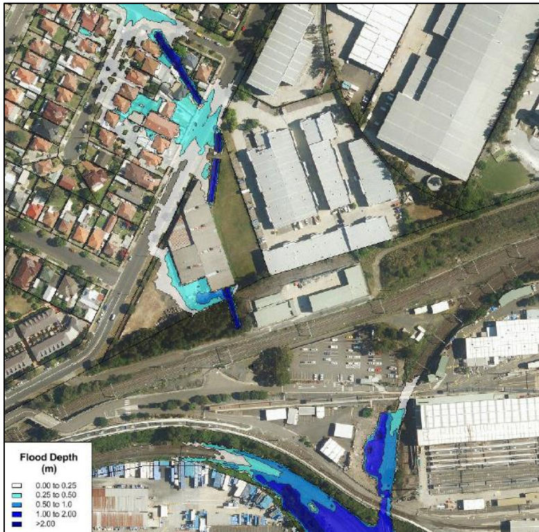
Figure 20: Existing conditions flood map 1% AEP Event (Source: Royal HaskoningDHV Flood Impact Assessment)
