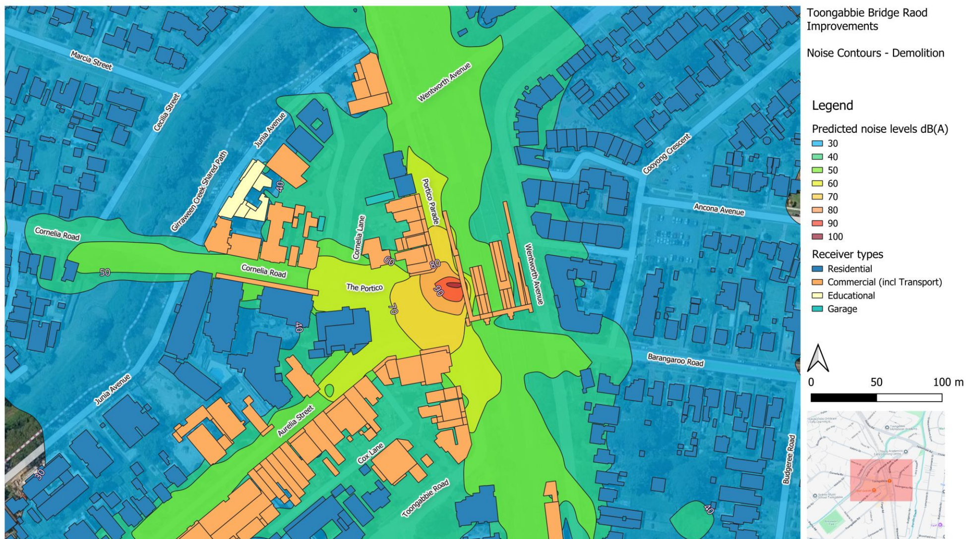
Figure 4-3 Noise Contours (All periods) L_{Aeq} – Site 5 demolition
