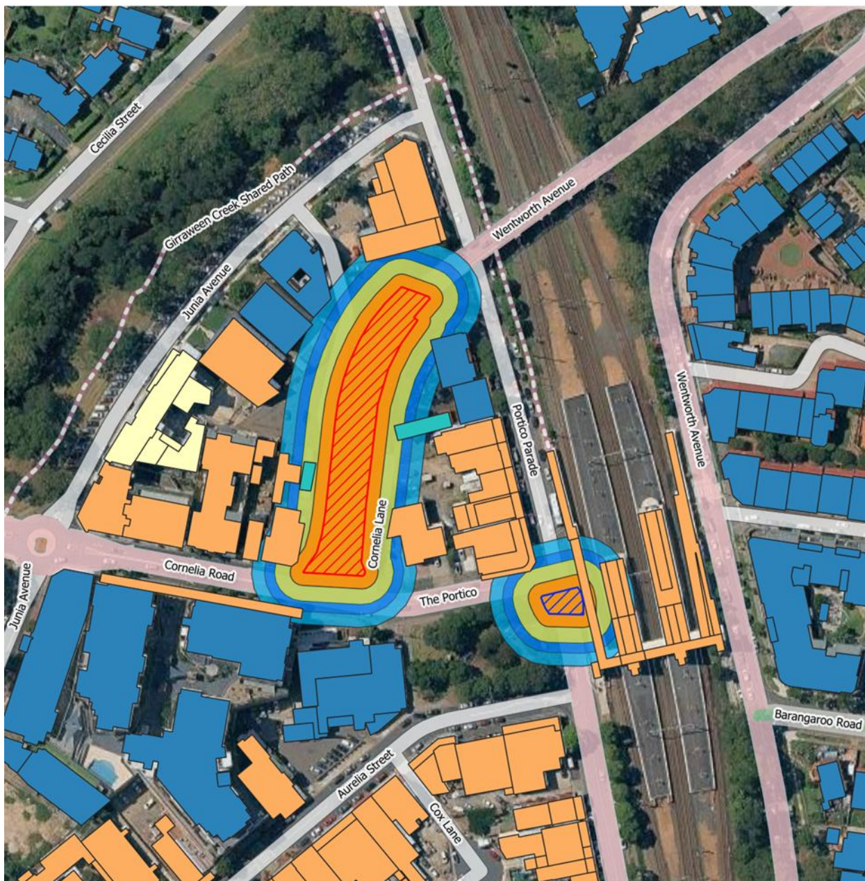
Figure 4-5 Minimum working distances for small roller for human comfort, heritage items and building damage
