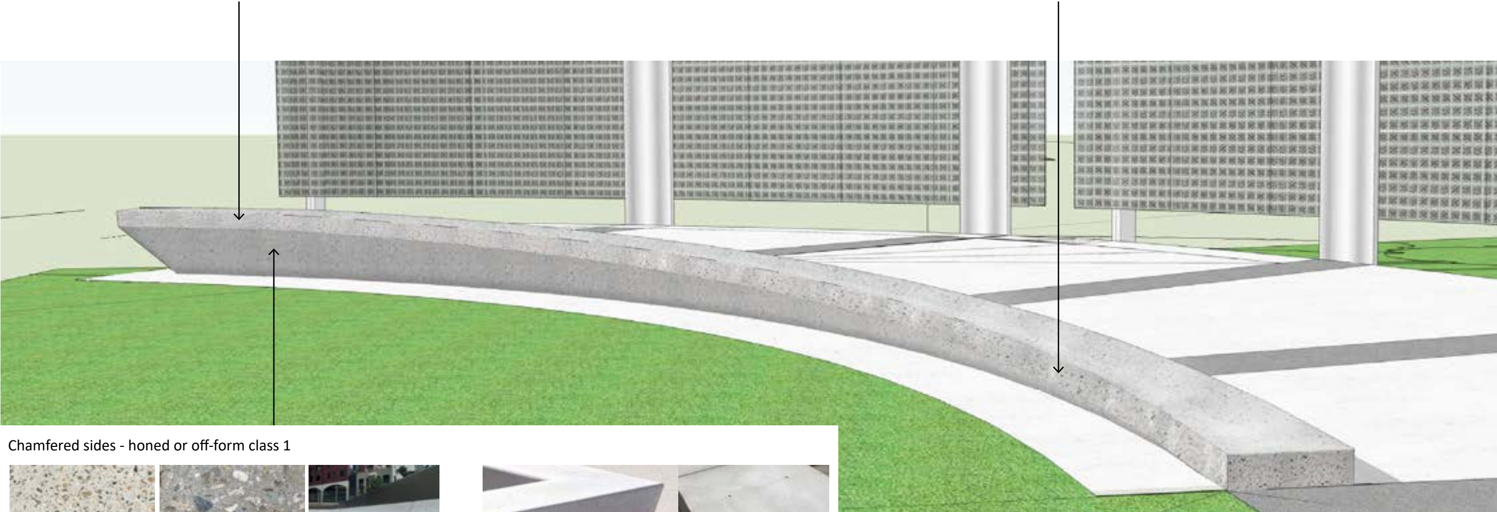
Wall top edge - polished finish or off-form class 1
