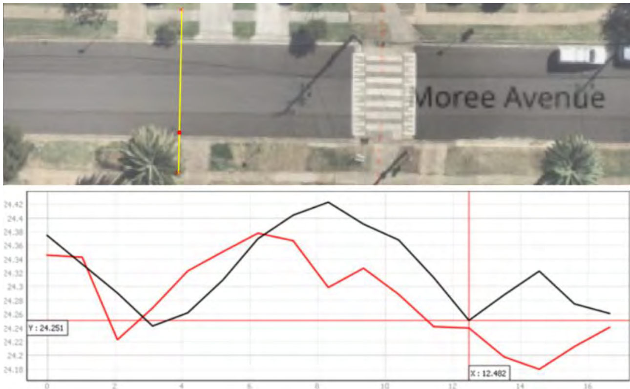
Diagram 7 – Ground Surface Elevation with cursor location corresponding to kerb & channel location (Black – 2013 LiDAR; Red – 2019 LiDAR)
