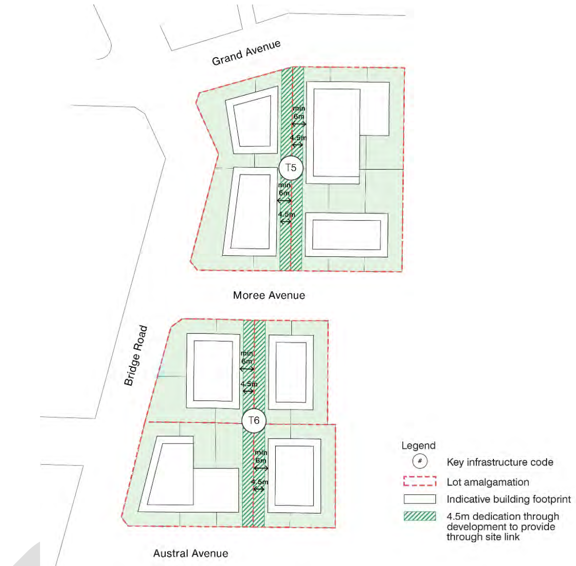
Figure 21. T5, T6 -Through site links between Austral Avenue and Grand Avenue – indicative plan
