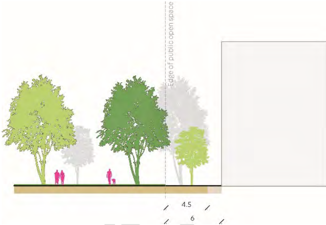
Figure 18. Publicly accessible link – showing intended 4.5m width of 6m typical setback buildings from boundary – widening of existing link or open space (right)
