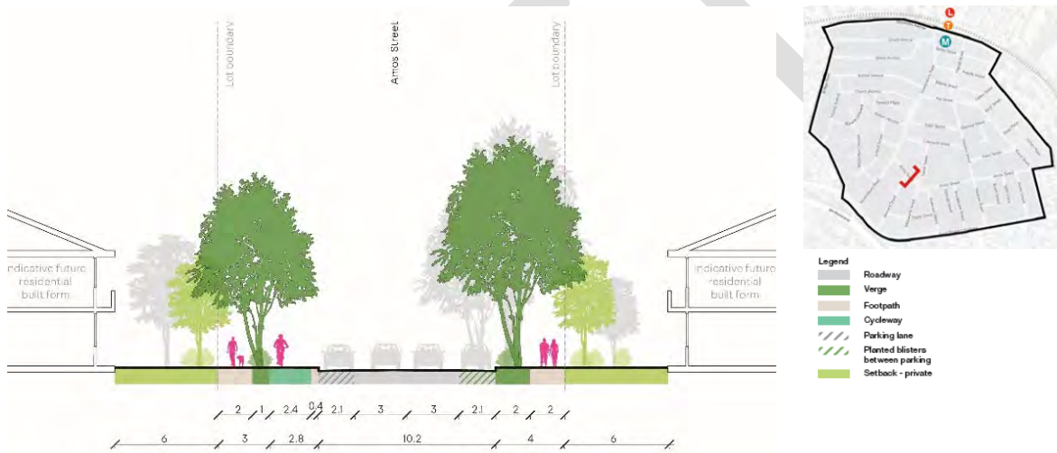
Figure 35. Amos Street typical section
