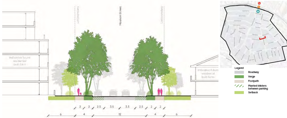
Figure 34. Hassall/Houison Street typical section
