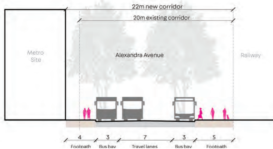
Street section (n.b. Additional width could be provided from either Metro site or railway)
