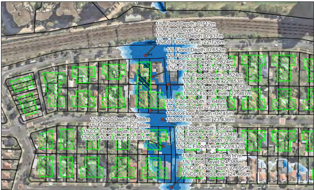
Diagram 17 – 1% AEP with Climate Change Flood Depths with Scenario 2 Buildings (Green) Overlayed at Grand Avenue, Westmead Creek
