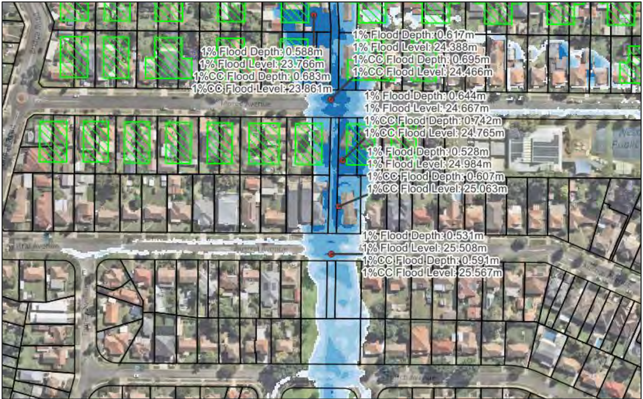
Diagram 18 – 1% AEP with Climate Change Flood Depths with Scenario 2 Buildings (Green) Overlayed at Austral Avenue, Westmead Creek
