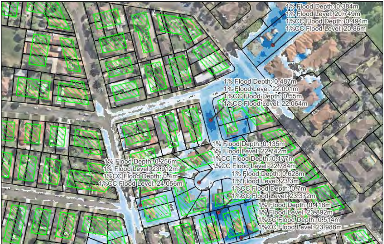
Diagram 20 - 1% AEP with Climate Change Flood Depths with Scenario 2 Buildings (Green) Overlaid at Thomas Clarke Street, Domain Creek
